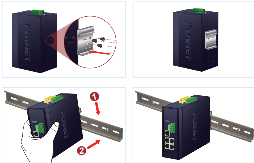
IFGS-620TF DIN-rail Mounting Installation
