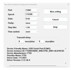
Figure 4-2: COM Port Configuration
