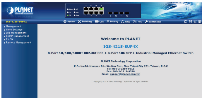
Figure 5-3: Web Main Screen of Industrial Managed Switch (Using IGS-4215-8UP4X as a representative)
