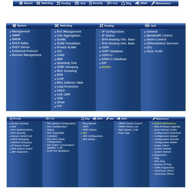
Figure 4-1-5: Managed Switch Main Functions Menu
