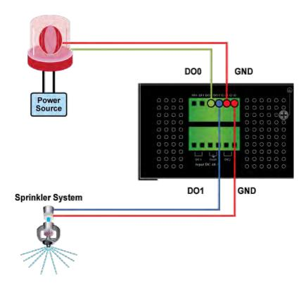
Figure 2-16: Wiring DO0 and DO1 to Open Detector
