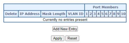
Figure 4-3-3-17: IP Subnet-based VLAN Membership Configuration page screenshot
