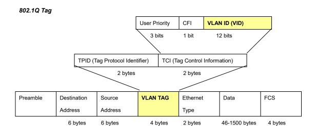
The Ether Type and VLAN ID are inserted after the MAC source address, but before the original Ether Type/Length or Logical Link Control. Because the packet is now a bit longer than it was originally, the Cyclic Redundancy Check (CRC) must be recalculated.
