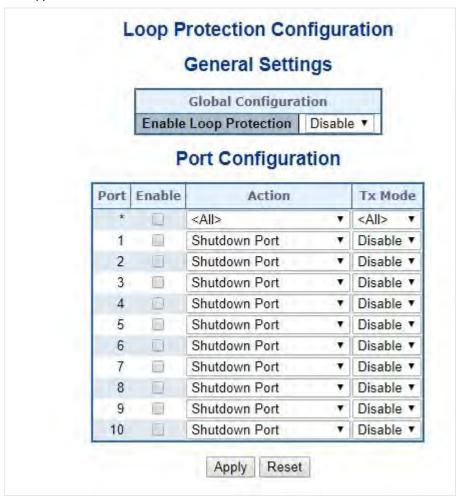
Figure 4-3-10-1: Loop Protection Configuration Page Screenshot
