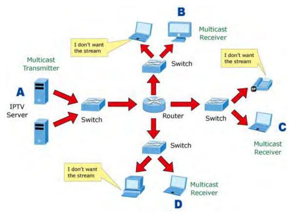
Figure 4-3-5-2: Multicast Flooding
