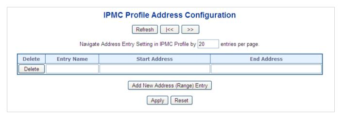
Figure 4-3-5-6: IPMC Profile Address Configuration Page
