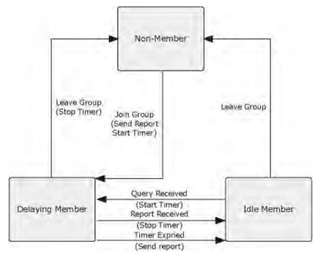
Figure 4-3-5-4: IGMP State Transitions
