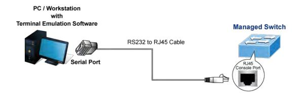
Figure 3-1: Industrial L2+ Managed Switch Console Connectivity
