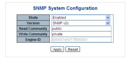
Figure 4-2-2: SNMP System Configuration Page Screenshot
