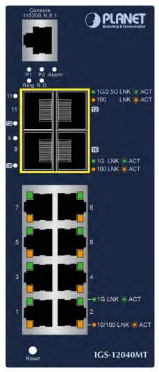
Figure 2-3: IGS-12040MT Switch Front Panel
