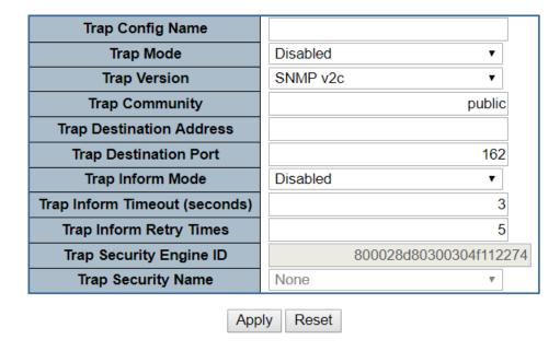
Figure 4-2-2-3: SNMP Trap Configuration Page Screenshot
