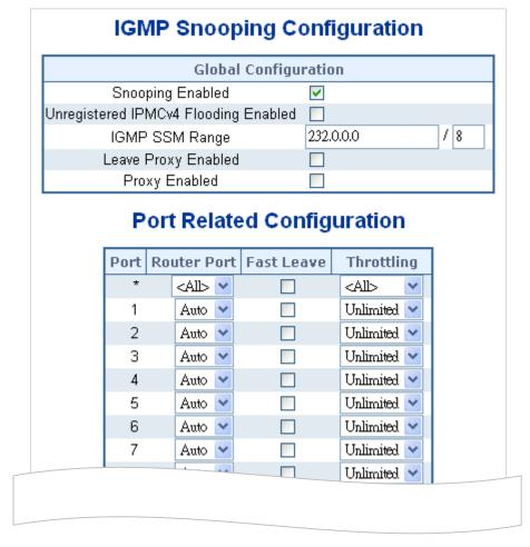
Figure 4-3-5-7: IGMP Snooping Configuration Page Screenshot
