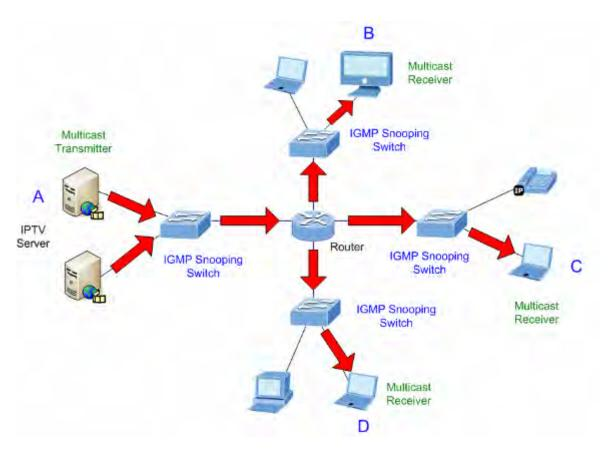
Figure 4-3-5-3: IGMP Snooping Multicast Stream Control
