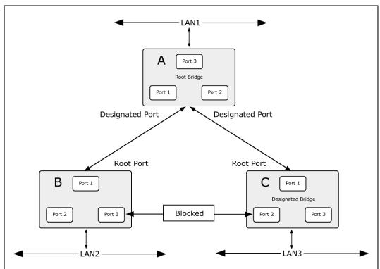
Figure 4-3-4-3: After Applying the STA Rules
