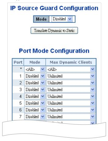
Figure 4-5-6-1: IP Source Guard Configuration Screen Page Screenshot
