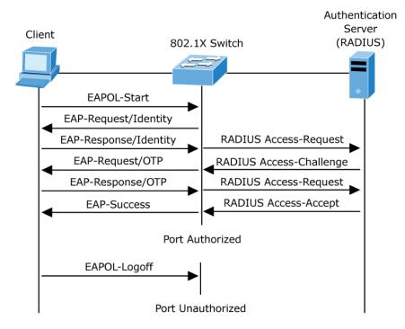
Figure 4-5-2-2: EAP Message Exchange
