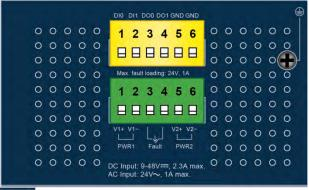
Figure 2-13: Wiring the Redundant Power Inputs
