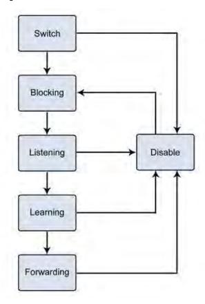
Figure 4-3-4-1: STP Port State Transitions
