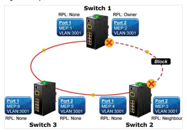
Figure 4-6-1-6: Ring Example Diagram
