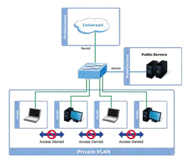
For private VLANs to be applied, the switch must first be configured for standard VLAN operation When this is in place, one or more of the configured VLANs can be configured as private VLANs. Ports in a private VLAN fall into one of these two groups:
