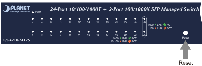
Figure 5-6: GS-4210-24T2S Reset Button
