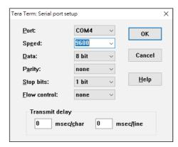
Figure 4-2 Tera Term COM Port Configuration
