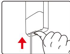
**Step 3:** Place the mounting strap through the slot on the back of the Outdoor Wireless CPE and then around the pole. Tighten the mounting strap to secure the Outdoor Wireless CPE.
