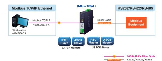
The advantage of having the IMG-210xT series is to assist users to build an industrial environment between the Modbus TCP/IP Protocol and the Modbus RTU/ ASCII Protocol easily, thus offering an application solution to the industrial control equipment without Ethernet ports and the industrial control equipment can only control through an industrial PC workstation or industrial control panel.
