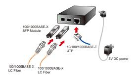
Figure 5: GT-1205A Gigabit Media Converter Standalone Installation
