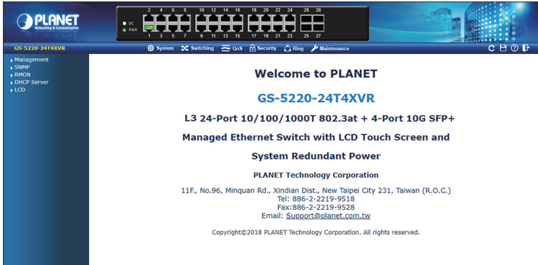
Figure 4-6: Web Main Screen of Managed Switch
