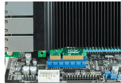
Step 5: If ENW-9740P is installed, please plug in firmly the **4 molex plug** from power supply.
