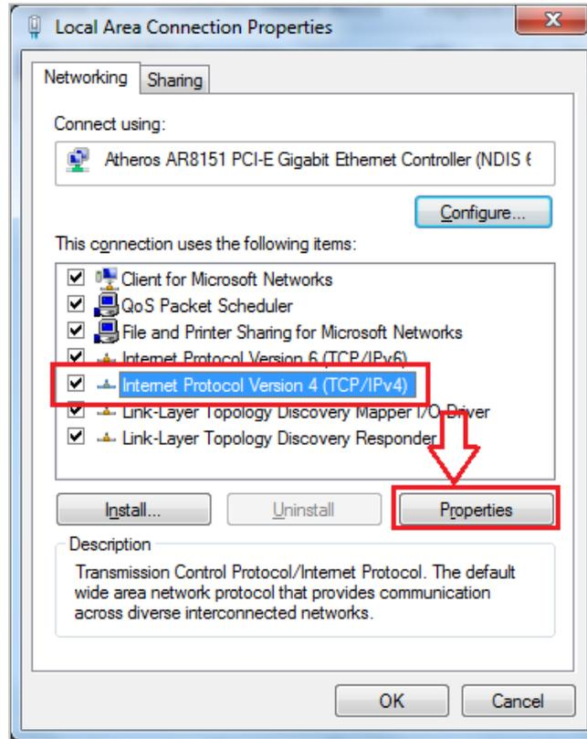
Figure 4-3 TCP/IP Setting
