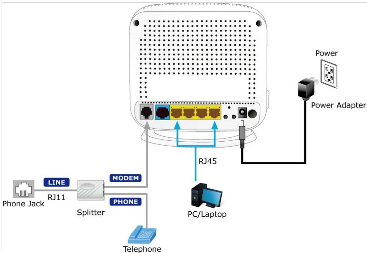
Figure 3-2 VDR-301N Connection Diagram
