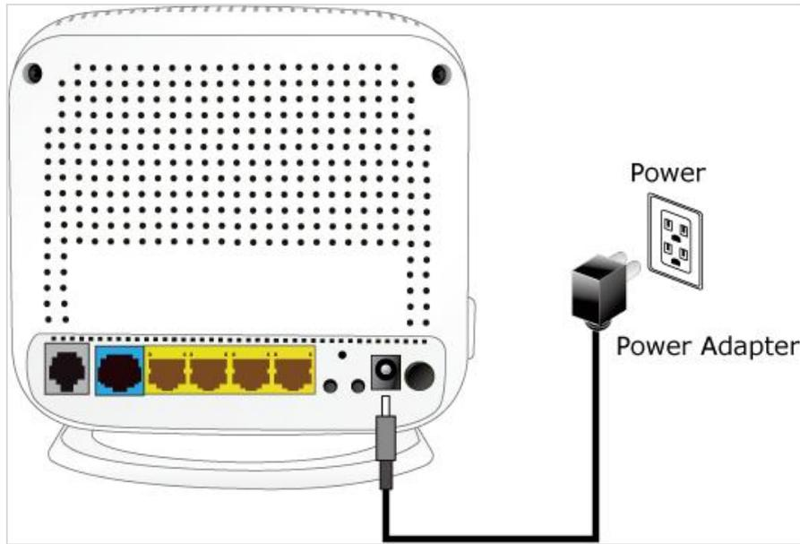
Figure 3-1 VDR-301N Power Adapter Connection Diagram
