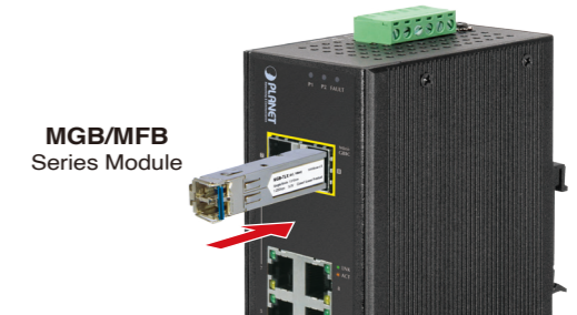
Figure 3-1: Plug-in the SFP Transceiver
