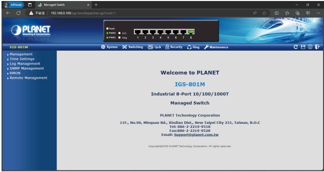
Figure 4-6: Web Main Screen of Industrial Managed Switch
