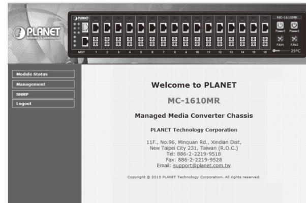
Figure 4-3: Web Main Screen of Managed Media Converter Chassis
