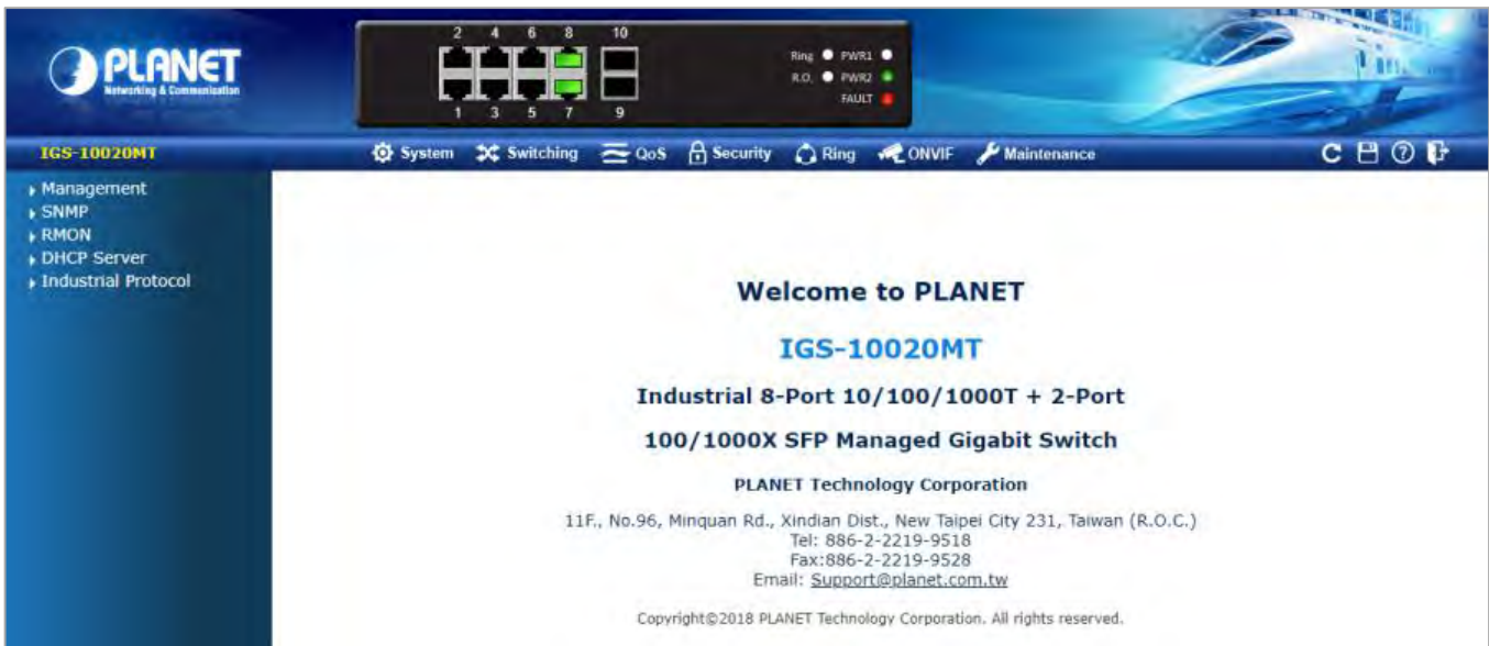
Figure 3-4: Web Main Screen of Industrial L2+ Managed Switch
