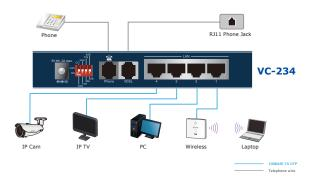
Depending on the quality of telephone line, the maximum distance of one VDSL segment is 1.4km (4593ft) with AWG 24 telephone wires. The distance could vary on the quality of telephone wires.
