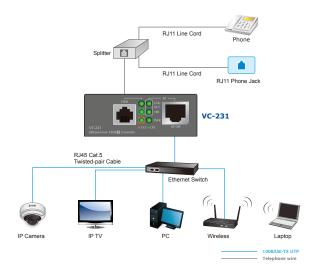
The VC-234 provides two RJ11 connectors for VDSL port. One for voice device connection (like telephone) and the other one for network link connection.
