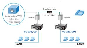
Refer to the following procedures to set up the VDSL2 Bridge LAN to LAN connection.
