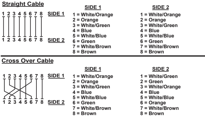
Figure A-1: Straight-through and Crossover Cable
