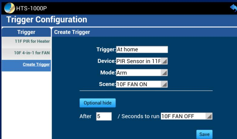
The screenshot shows the 'Trigger Configuration' screen for HTS-1000P. It includes a table with triggers like '11F PIR for Heater' and '10F 4-in-1 for FAN'. The 'Create Trigger' form is filled with: Trigger: At home, Device: PIR Sensor in 11F, Mode: Arm, Scene: 10F FAN ON. An 'Optional hide' section is set to 'After 5 / Seconds to run 10F FAN OFF'. A 'Save' button is at the bottom right.
