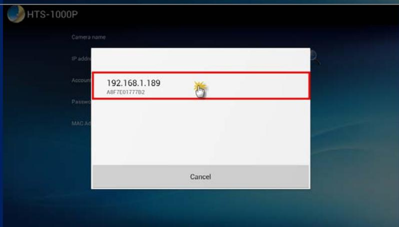
Fill out the command line and MAC address of camera automatically.
