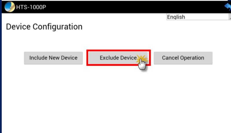
When you see the message of "Waiting for user action", you can press the match button on Z-Wave devices to exclude device.
