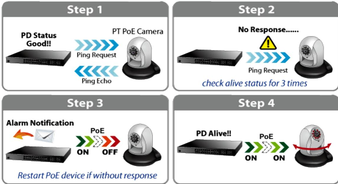
This page provides you with how to configure PD Alive Check. The screen in Figure 4-16-10 appears.
