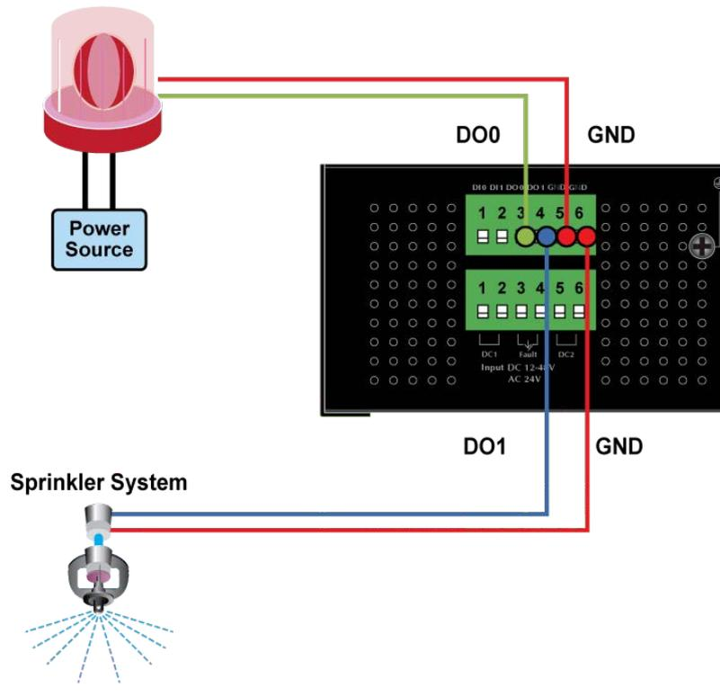
Figure 2-22 Wires DO0 and DO1 to Open Detector
