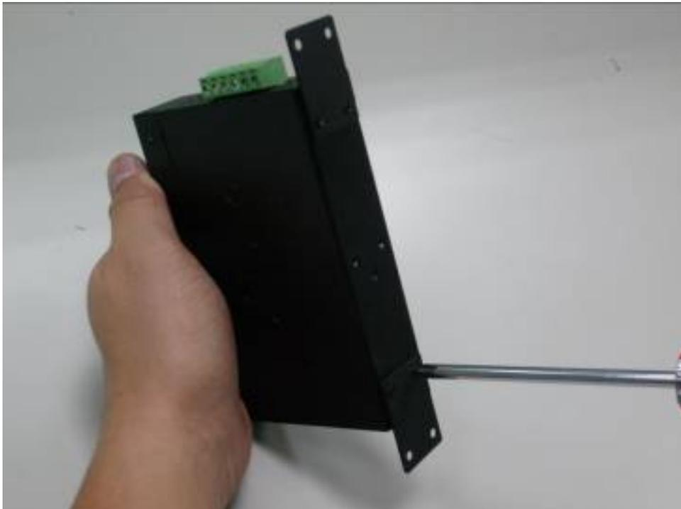
**Step 3:** Use the screwdriver to screw the wall mount plate on the **Industrial Managed Switch**.
