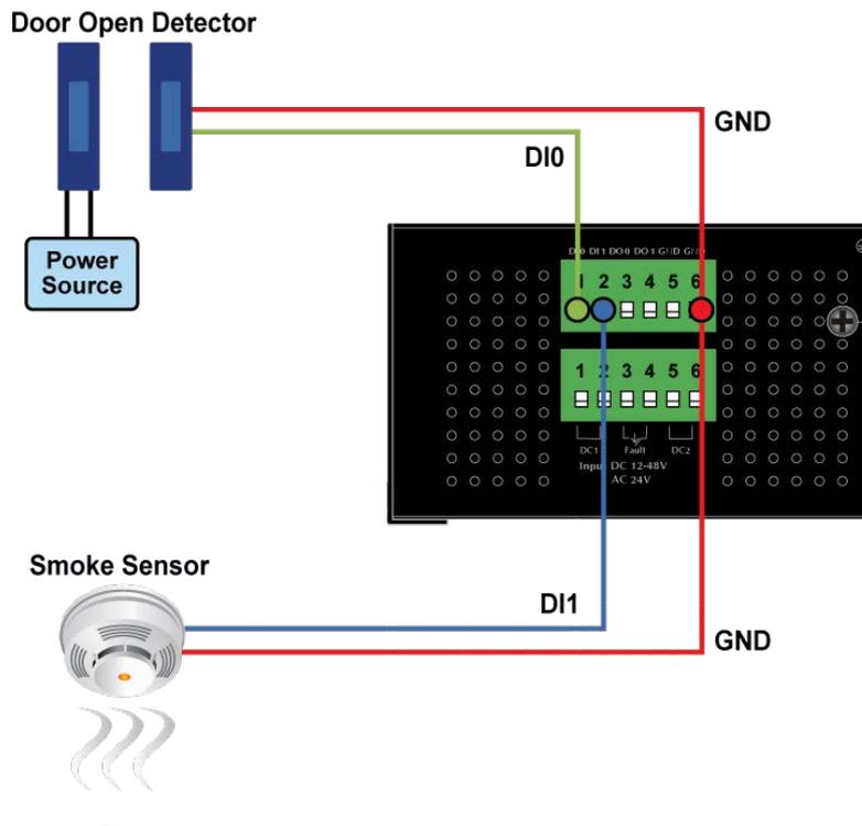
Figure 2-21 Wires DI0 and DI1 to Open Detector
