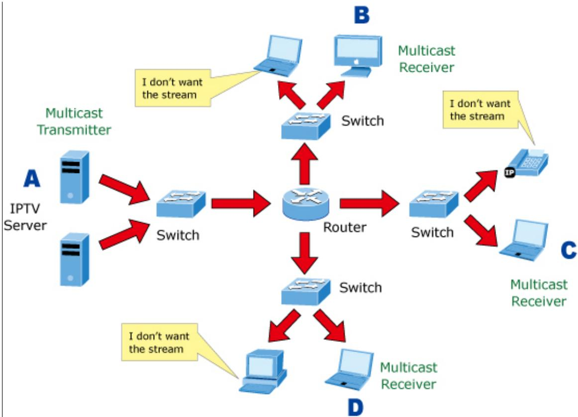
Figure 4-8-2: Multicast Flooding
