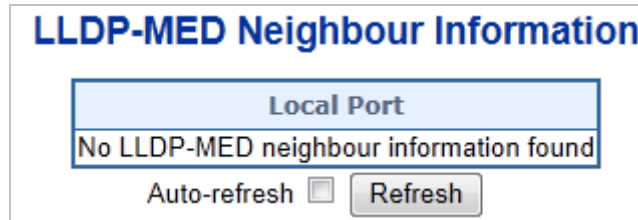
Figure 4-14-3: LLDP-MED Neighbor Information with no LLDP-MED device detected
