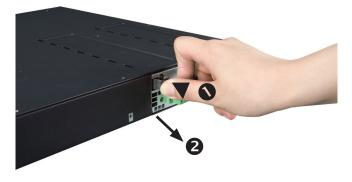
Figure 5-1 Removing the XGS3-PWR150-48
